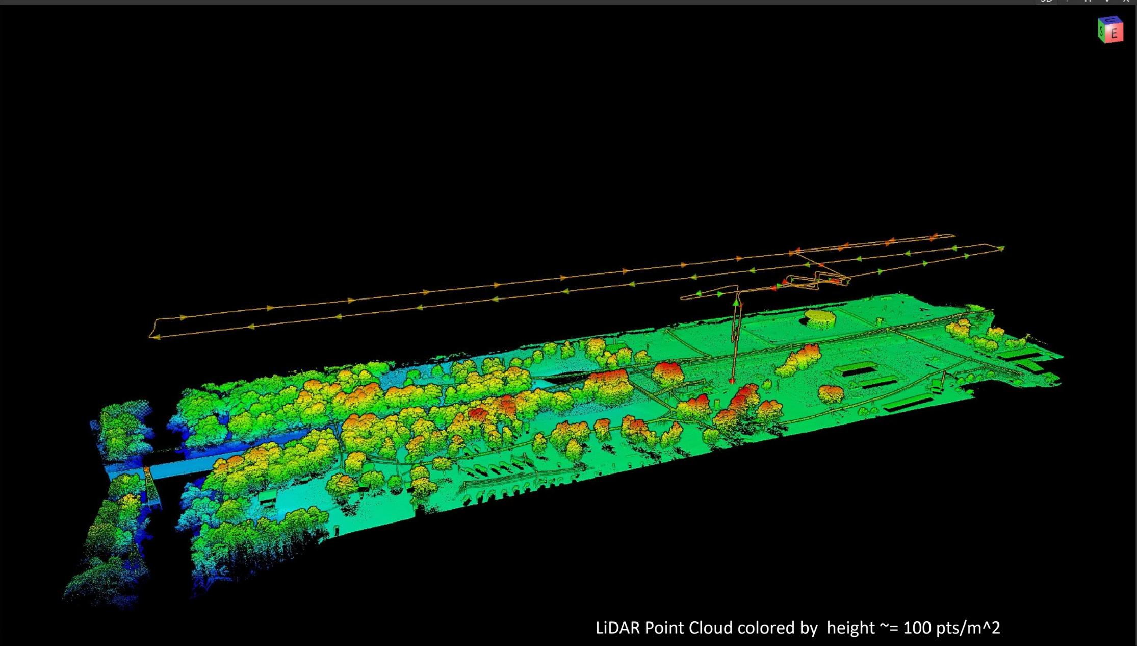
LiDAR Point Cloud colored by height  $\approx 100 \text{ pts/m}^2$
