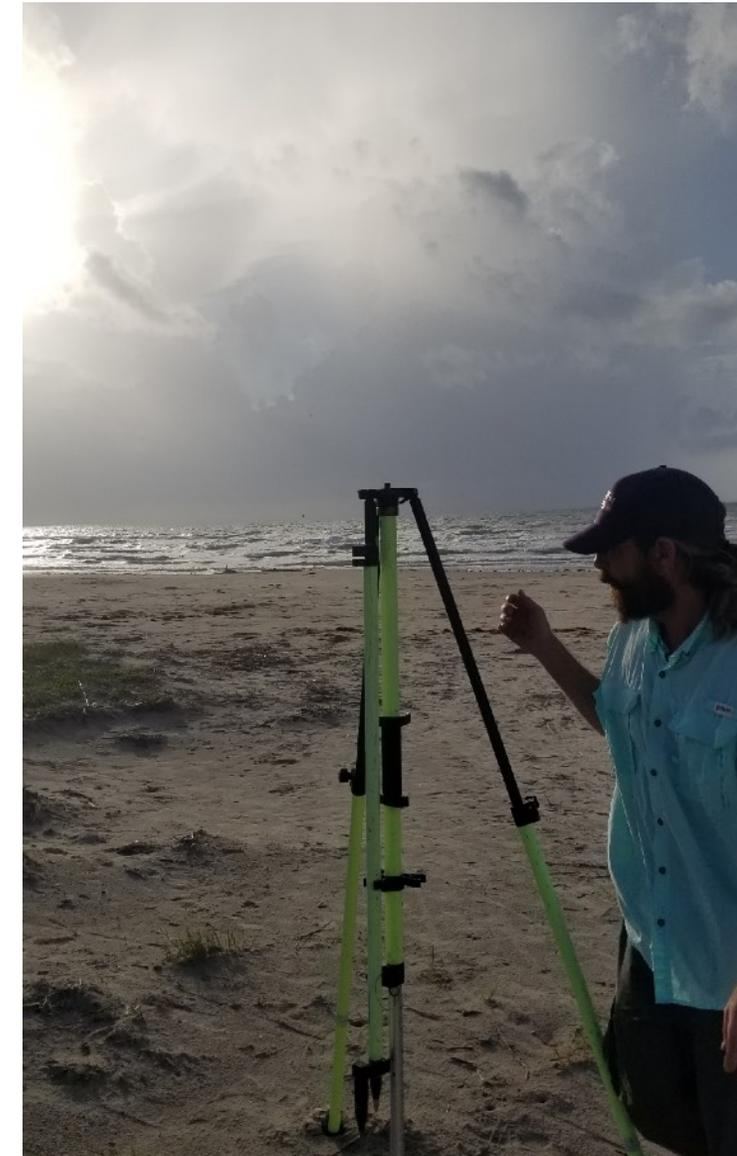
Establishing static setup for local base at MISP
