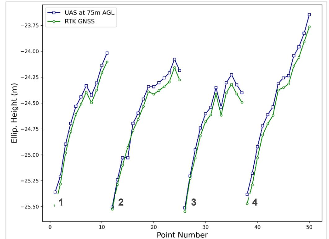
Height profiles [UAS vs RTK GNSS]
