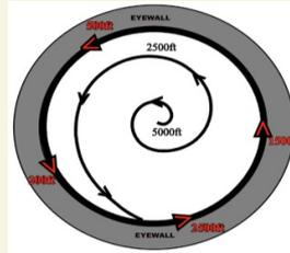
**Inflow Module:** Provide sUAS HDOBS in near-real-time to NHC for visualization in AWIPS II. Post storm, compare sUAS TC boundary layer thermodynamic, kinematic and SST radial structure to improve TC boundary layer parameterizations and ocean response in HWRF and HAFS.
