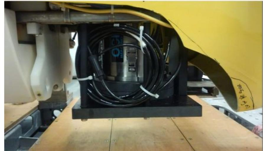
Fornari 20mpx camera installed aft end of Sentry
