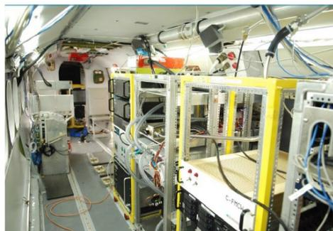
**Cabin:** Nephelometer, Sootphotometer, CPCs, UFCPC, Data System Racks for ‘Research’ and ‘Guest’ Instruments. Satcom system
