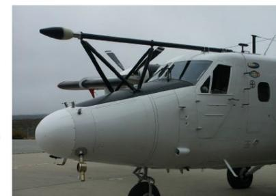
**Nose:** Temperature, Dew Point, Pressure (Static, Dynamic Sideslip Attack angle), GPS/INS, IR Temperature, Liquid Water Content, Aerosol Inlet
