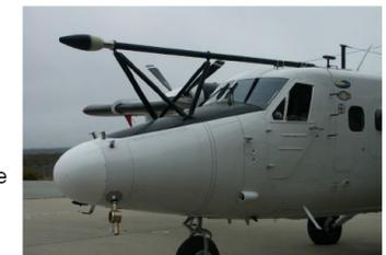
**Nose:** Temperature, Dew Point, Pressure (Static, Dynamic Sideslip Attack angle), GPS/INS, IR Temperature, Liquid Water Content, Aerosol Inlet
