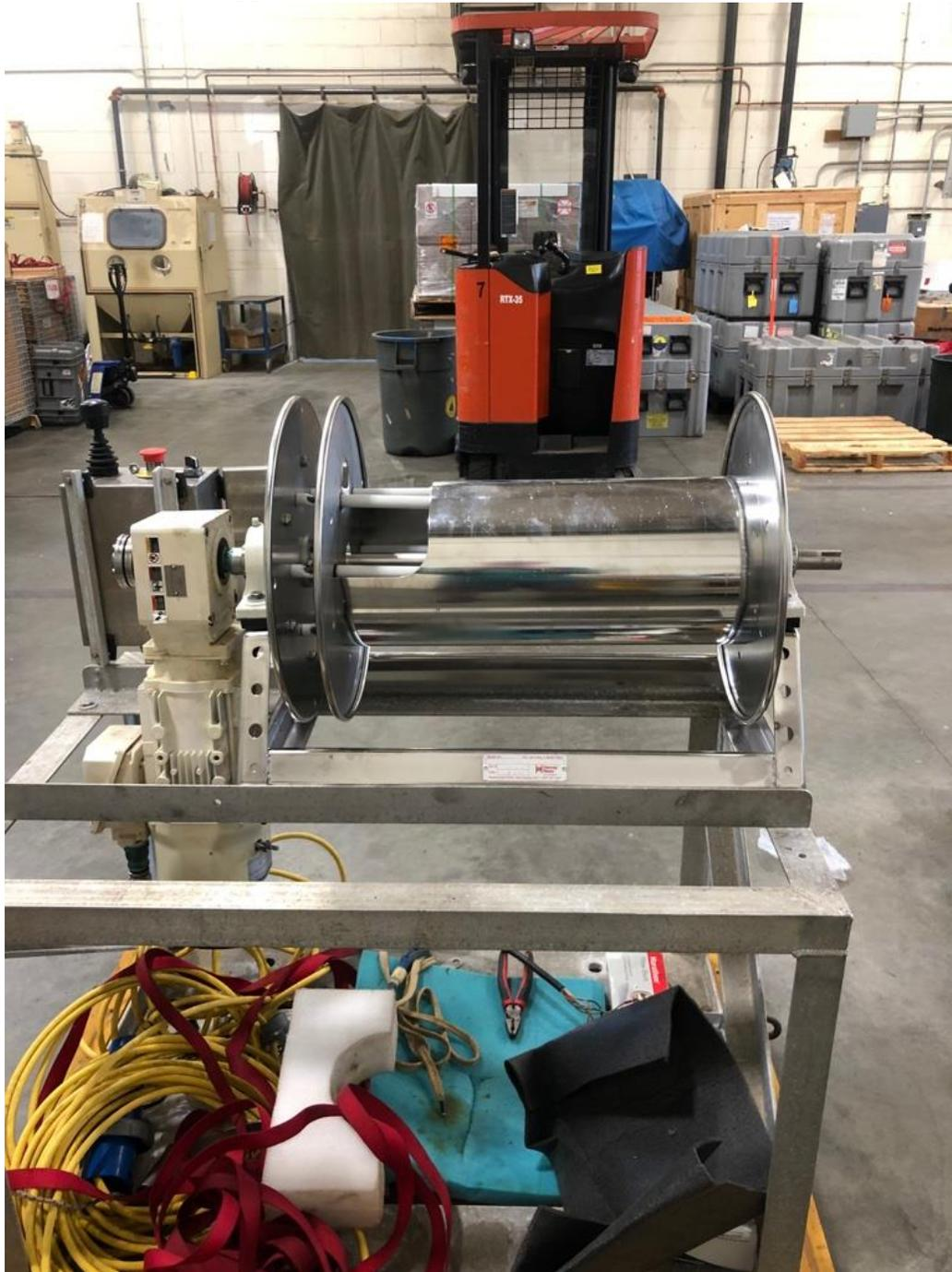
Refurbished magnetometer winch (1 of 2) for SeaSpy 1 and 2 maggie systems
