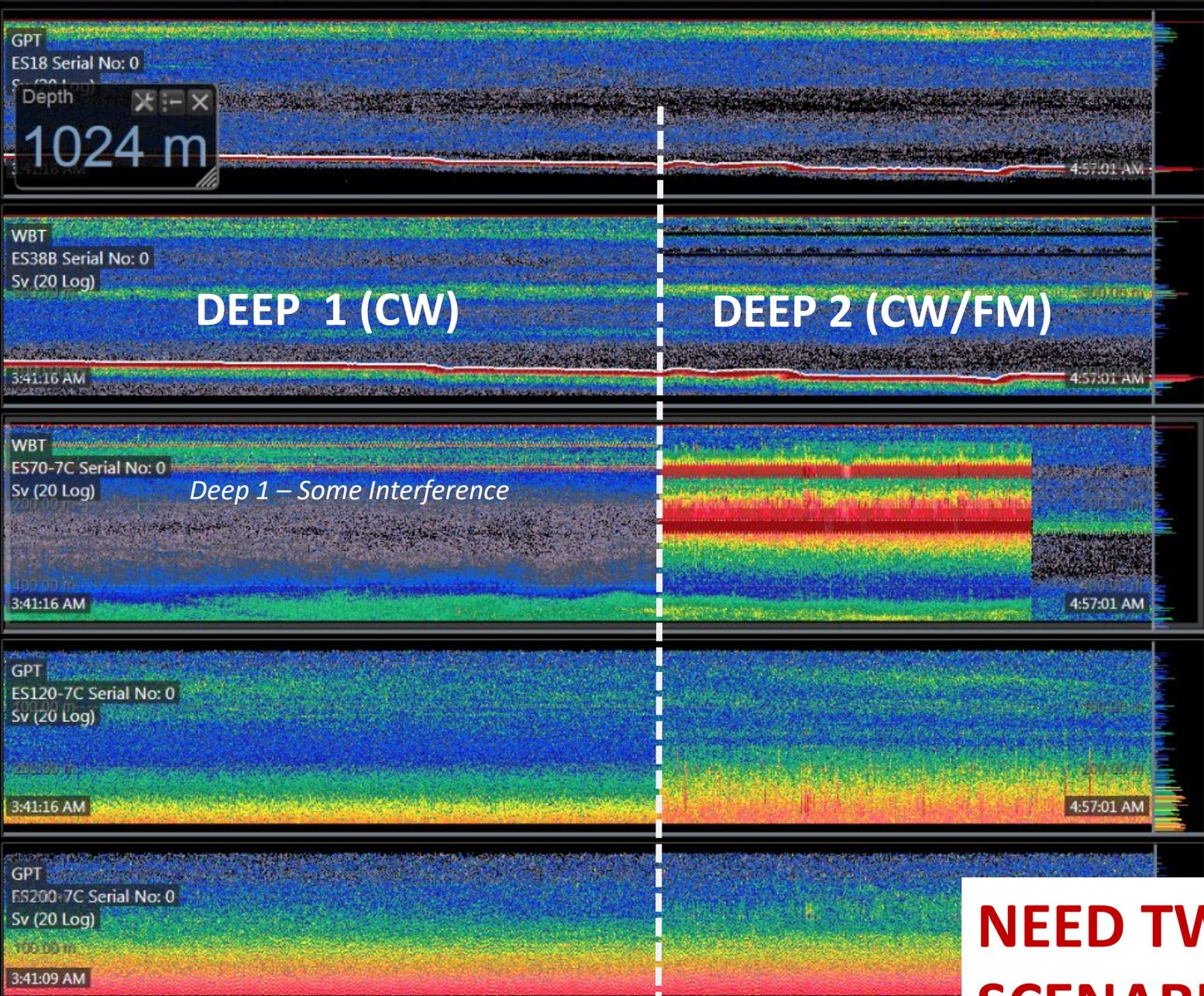
*Effect on EK water column data from the EM 302 changing between CW and FM mode when it moves from DEEP 1 to DEEP 2 at ~ 1000 m*
