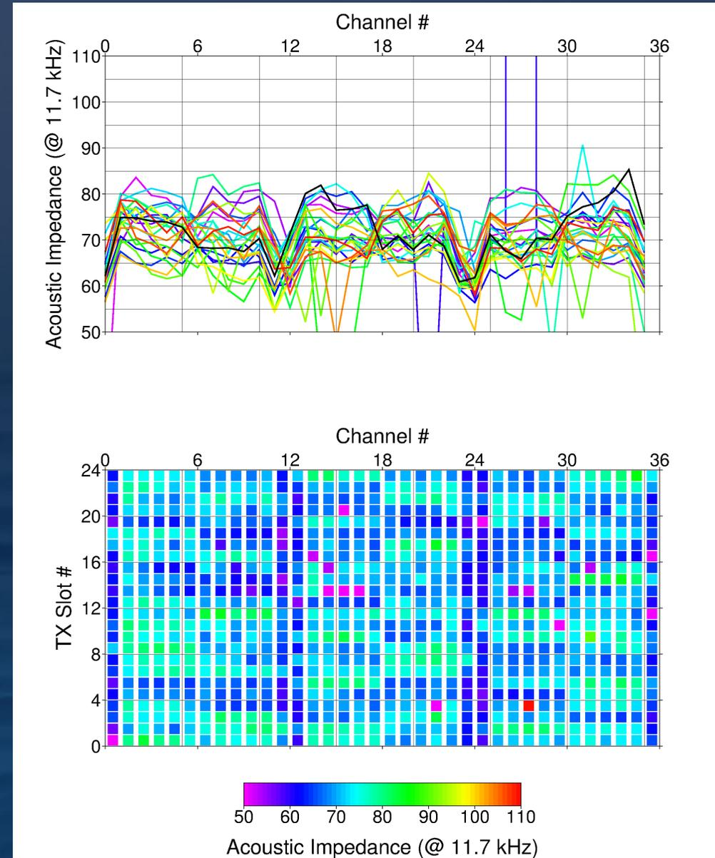
12-kHz TX array after 10 years of icebreaking
