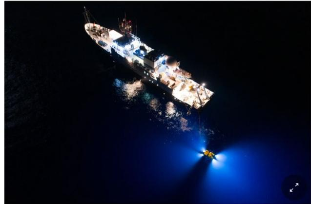
The Nautilus, a research vessel, towing an underwater remotely operated vehicle that was used to hunt for the airplane of Amelia Earhart, which disappeared in 1937. Robert Lyall/National Geographic
