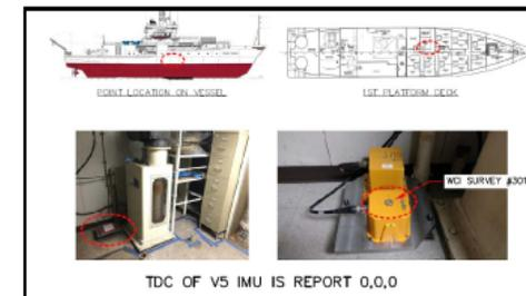
Figure 2. The most useful and intuitive origins described in survey reports are unambiguous, durable, physical markers that are accessible at any time. This example survey origin is a clear, permanent target on the motion sensor housing that is conveniently co-located with the origin chosen for mapping system configuration. (Image: Westlake Consultants, Inc.)
