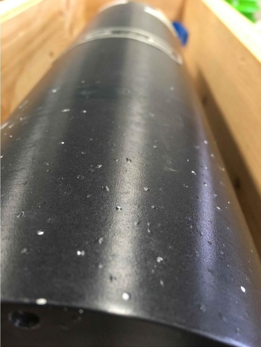
The SIO MPL machine shop investigated the cause of the pitting and suggested that there may have been something wrong with the batch of 7075 material that the cases were made from. 7075 is an aluminum/zinc alloy and if the zinc component had migrated to the surface due to either faulty material or improper heat treating or anodizing then it could result in pitting.
