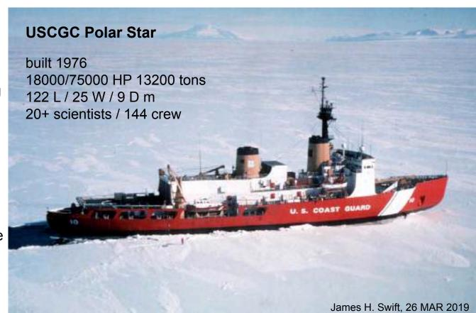
Icebreaking capability is needed to support both Arctic and Antarctic marine research.
