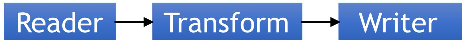
Read from serial port, prefix with timestamp and instrument id, write to file
