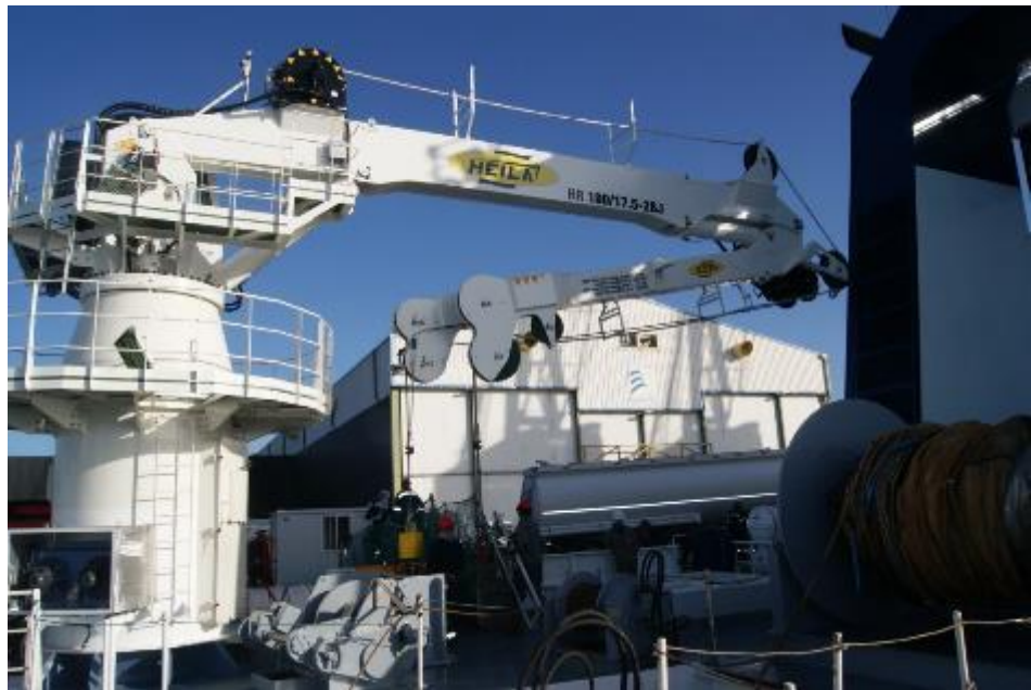
New oceanographic HEILA knuckle crane 180t.m – 2 winches (4t & 13t) – 20m at full extension
