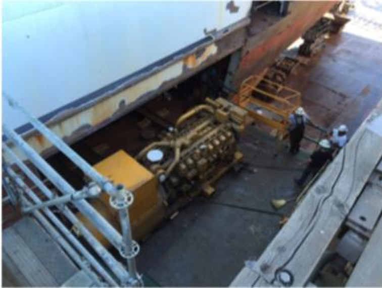
First Generator being removed in dock through side of lower engine room
