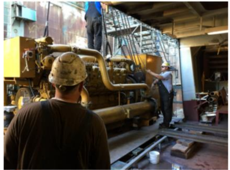
First Generator being removed in dock through side of lower engine room
