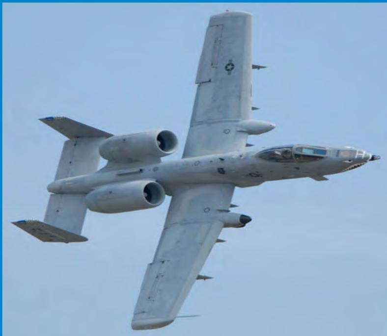
A-10 has 11 hard points on wings and belly where 8000 lbs of instruments may be suspended.
