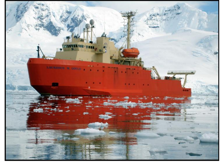
R/V Lawrence M. Gould ECO contract w. NSF Antarctic contractor constructed 1997 3780 tons / 4575 HP 70 L / 14 W / 6 D meters
