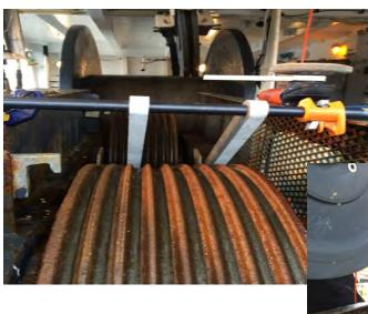
Reconditioning of Endeavor's traction heads
