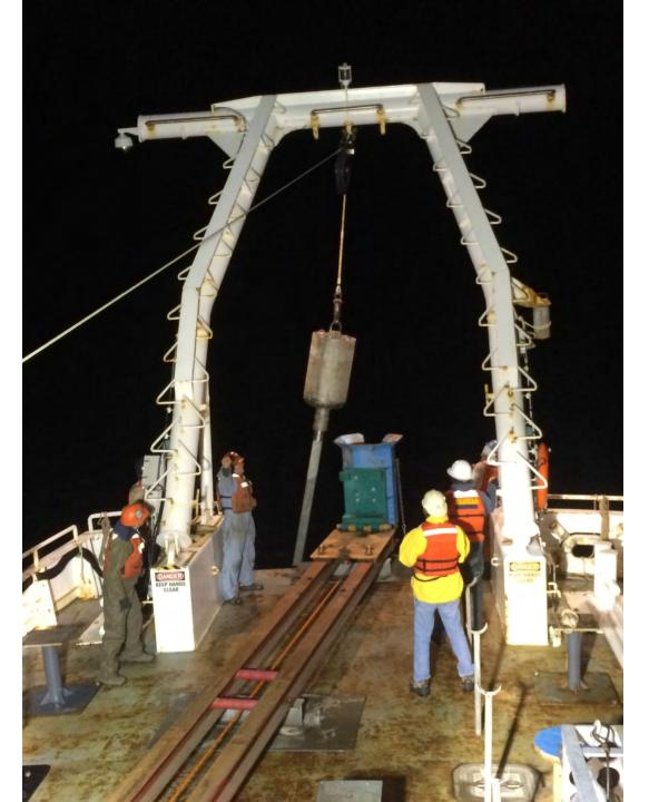
Rope configuration following the first coring operation after being disconnected from the core head.
