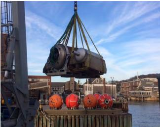
Load Tests using the Armstrong's Traction winch and lifting 20,000 lbs.
