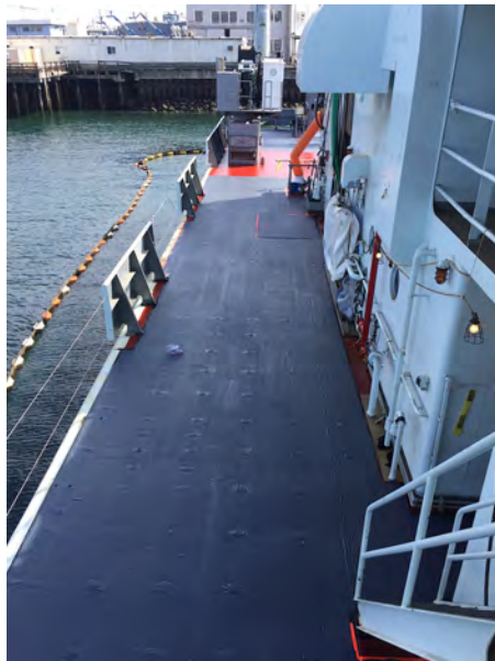
Blasted/Painted working decks
