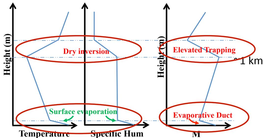
**Negative moisture gradient layers result in trapping of EM waves.**
