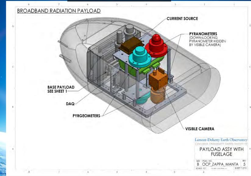
BASE payload allows for quick change between sensor payloads
