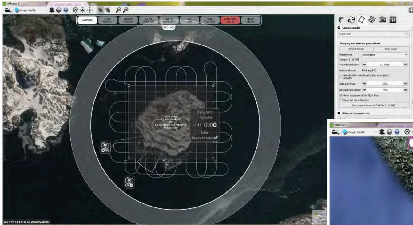
Flight plan for typical Torgerson Island fixed wing UAS survey
