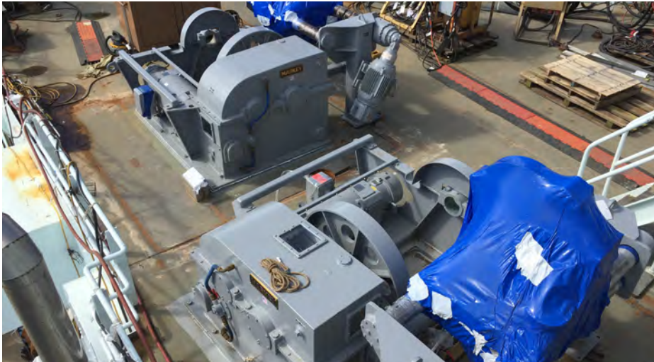
Refurbished hydro-winch in place
