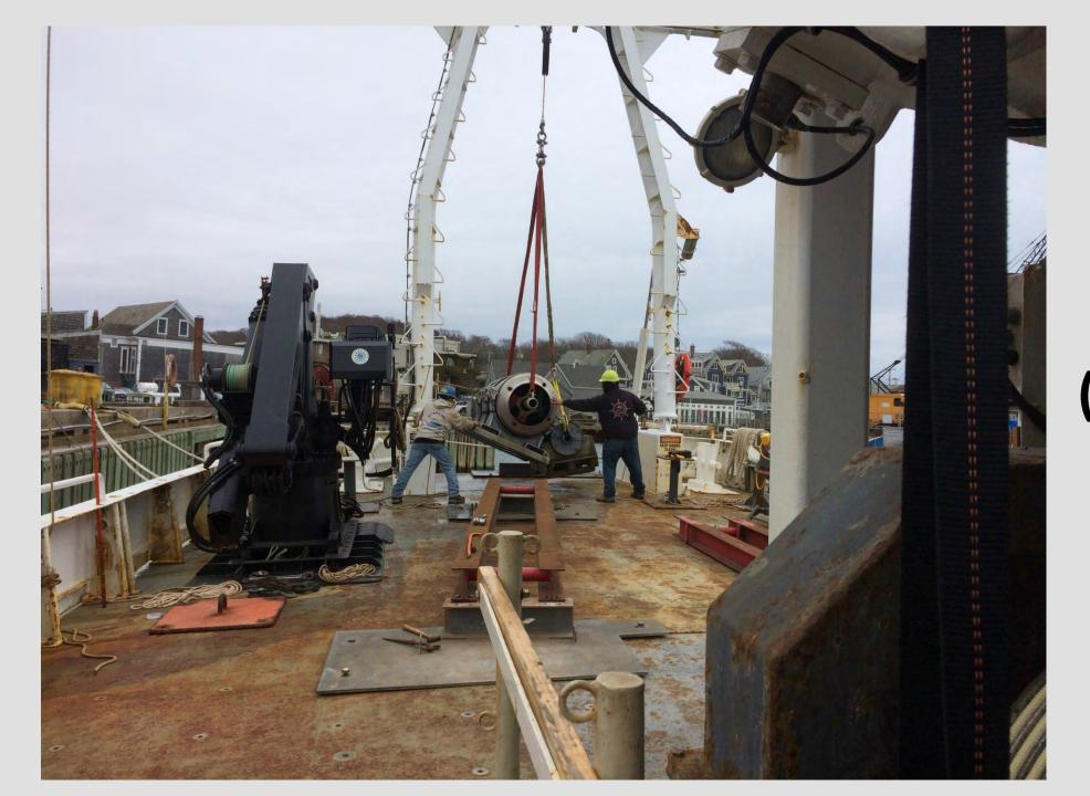
6,804 kg (15,000 lbs.) Load Test Phillystran product wound onto the winch and load tested, lifting 2,268, 4,536 and 6,804 kg successfully.
