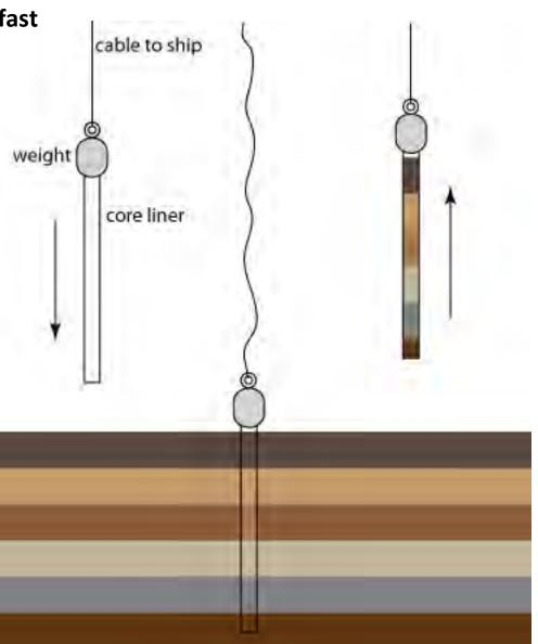
Gravity corer is pulled out of the bottom with sediment sample.
