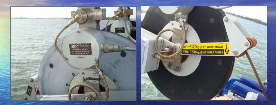
RV SAVANNAH: Instrument blocks that measure the wrap angle in order to measure the tension in the cable.
