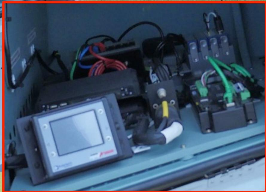
The Quadruple Eddy Correlation System for the calculation of turbulence variables and, in particular, momentum, heat, and mass turbulence fluxes. Also possible is the detection of gravity waves from approaching hurricanes (?)
