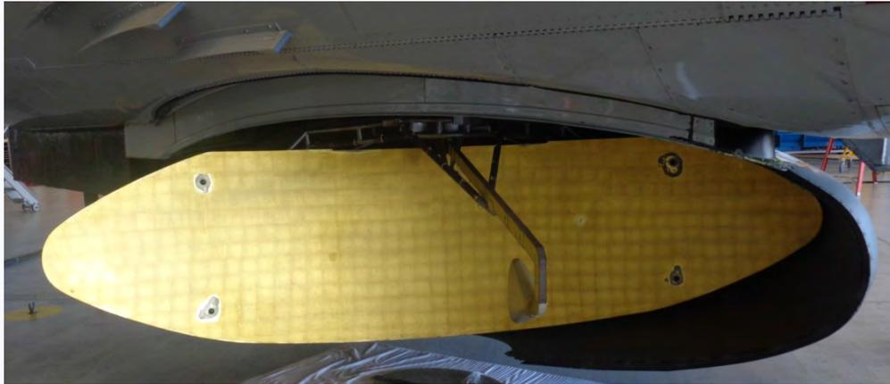
Replace Lower Fuselage Weather Radar with AN/APY-11 Multimode Radar System
