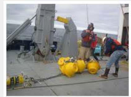
The Tasman team uses moorings like this one that typically include dozens of temperature sensors at varying depths, and multiple current profilers and conductivity, temperature, depth (CTD) profilers. Credit: Amy Waterhouse
