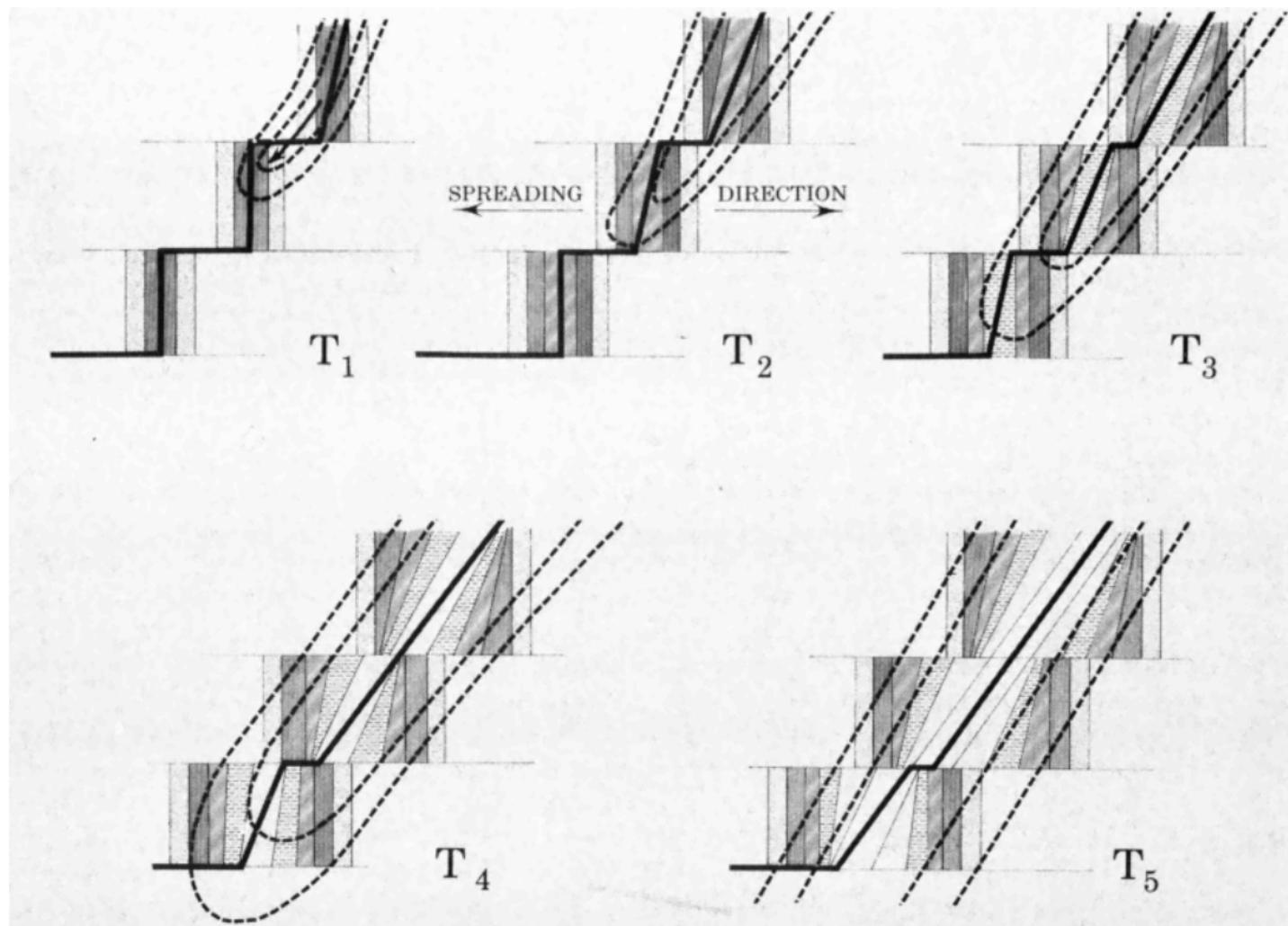
Vogt & Johnson (1975) reorganization model, in which Iceland plume asthenospheric flow (dashed contours) thermally weakens axial lithosphere & progressively rotates each segment by differential asymmetric spreading, creating a sequence of "zed pattern" reorganizations (e.g., Menard & Atwater, 1968).
