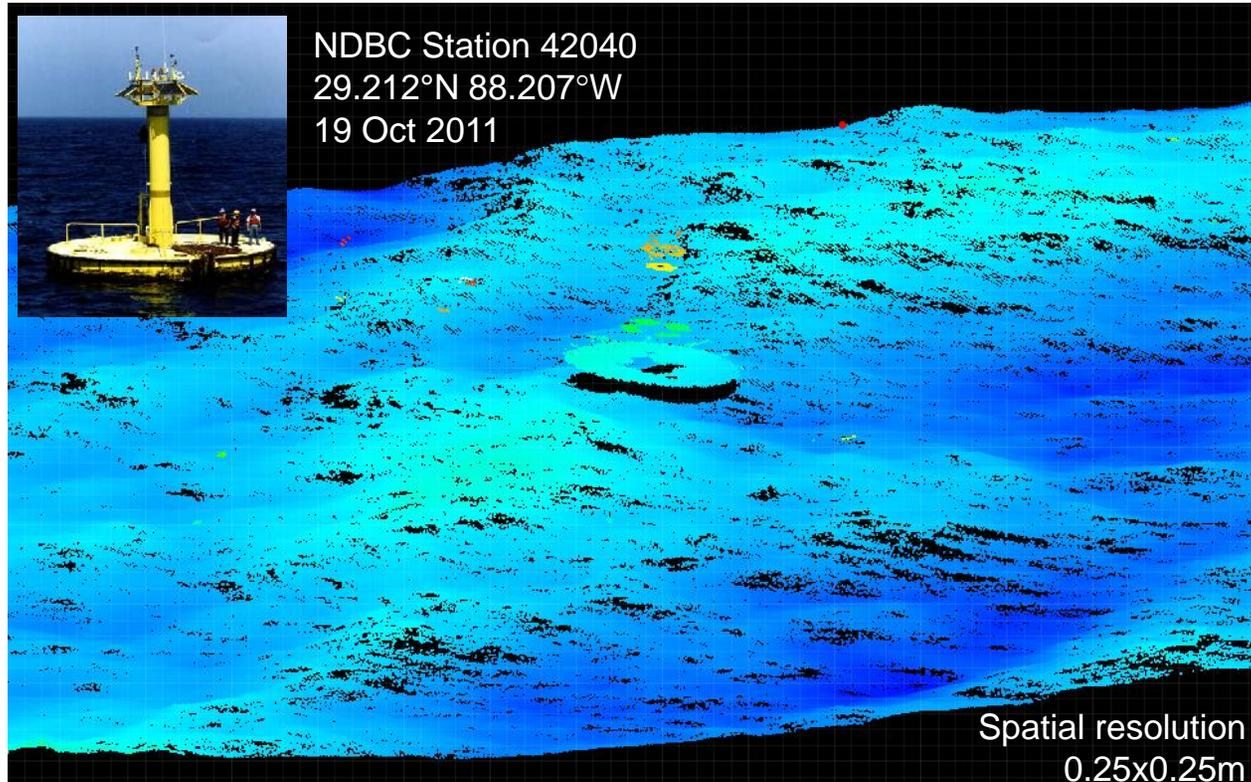
*Example of surface elevation as measured from the MASS during a recent experiment in the Gulf of Mexico, flying above NDBC buoy #42040. (wind~12m/s, Hs = 3.1m)*
