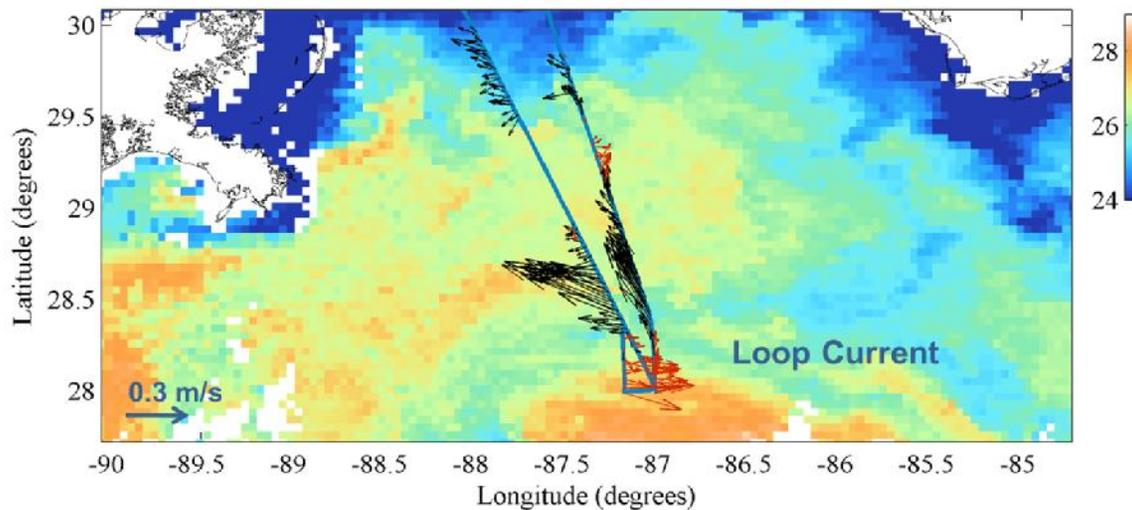
Sea surface temperature estimated from TERRA level 3 daily product ( $^{\circ}\text{C}$ ) on October 30, 2011, 10hr prior to the airborne survey conducted the same day. The flight track is shown in blue. The average surface velocities derived from the thermal imagery are shown as vectors along the flight track (red, positive easterly velocity, black, positive westerly velocity). Note the sharp change in surface velocities as the aircraft went across the LC.
