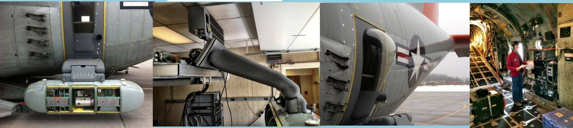
**Figure 2** IcePod Components IcePod Common Science Support Pod (CSSP) (far left), SABRE arm (center left), Door plug (center right) and Instrument rack (left)
