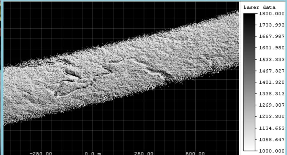
Figure 3 Riegl VQ-580 airborne laser scanner and swath elevation over a Greenland melt channel
