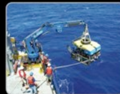
Figure 1 (above). ROV Jason, part of the UNOLS National Deep Submergence Facility operated by Woods Hole Oceanographic Institution. Photo credit: Tom Bohlen, Woods Hole Oceanographic Institution
