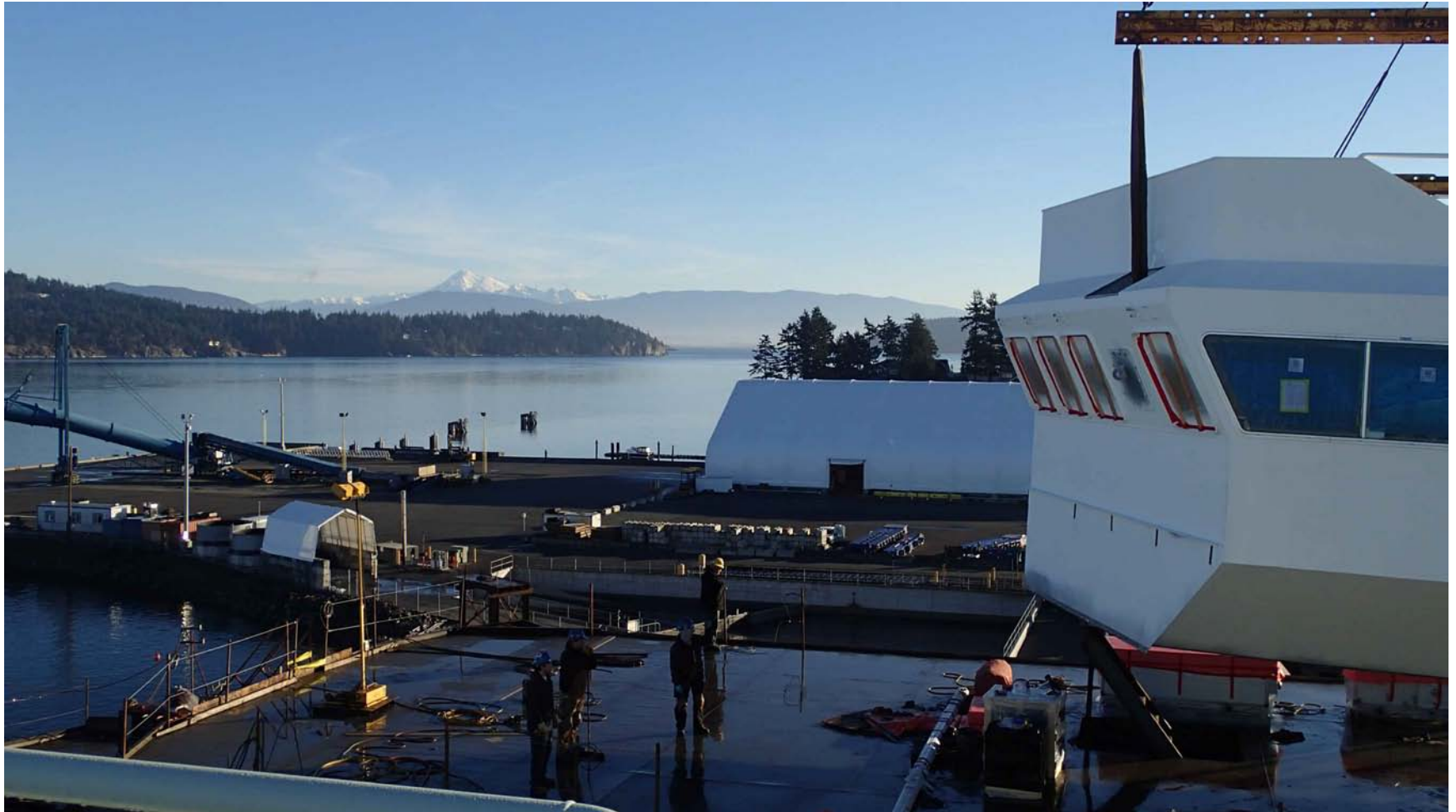
Pilot house being landed on Sally Ride
