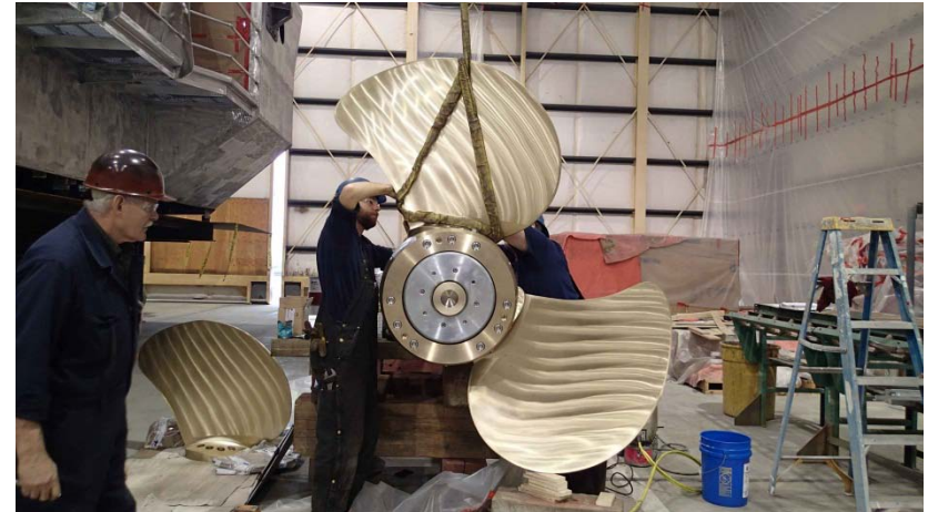
Controllable Pitch Props being assembled
