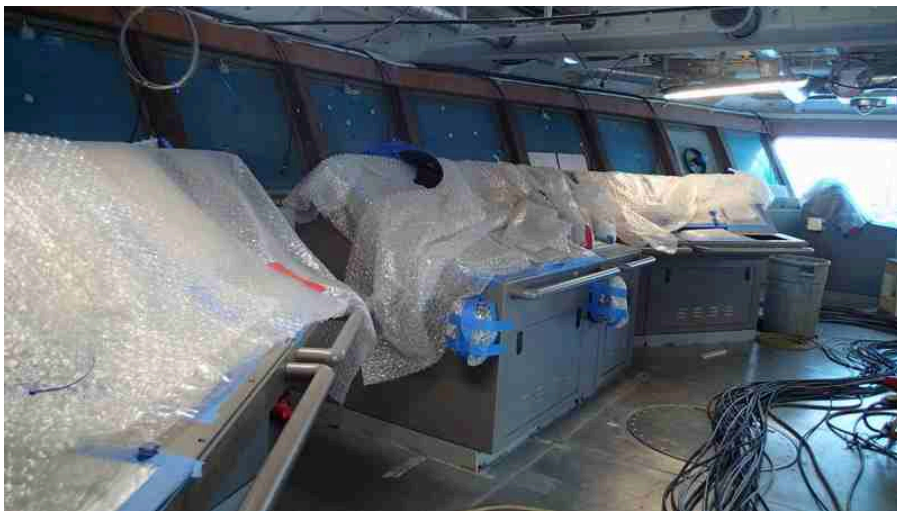
Bridge Consoles being installed
