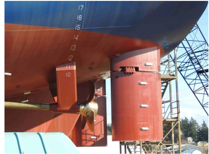
Paint, Zincs, Ready to Float
