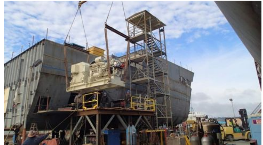
Cummins Genset loaded into AGOR 27
