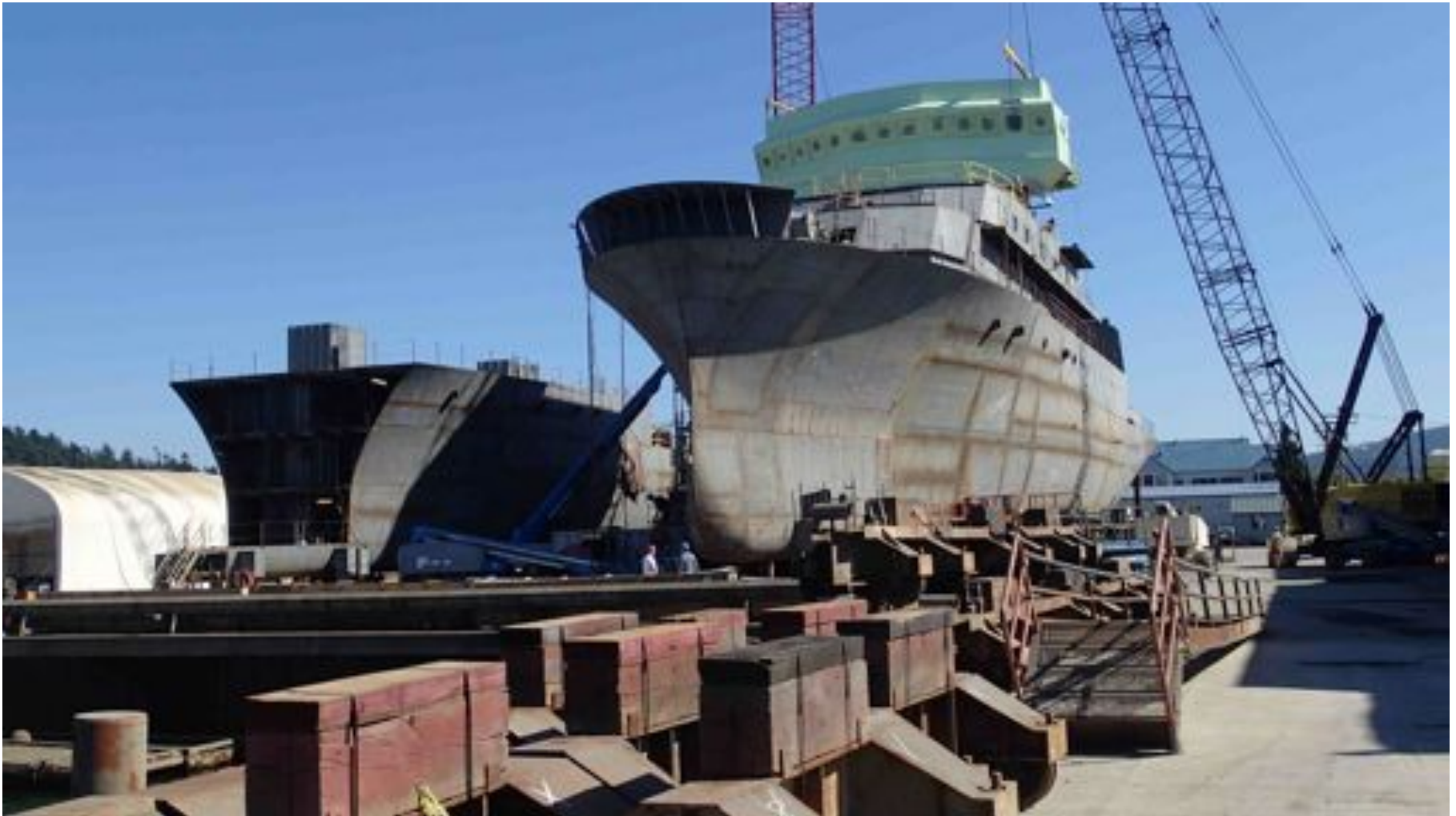
Pilot House being installed on Neil Armstrong
