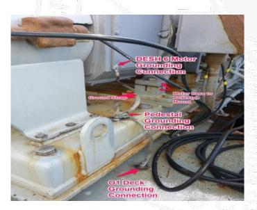
Built-up paint and corrosion on the winch pedestal were to blame for the inadequate ground.
