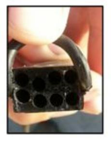
One of the issues we faced this year was with the ADCP cables to ADCP top hat connection. Our group experienced a set of leaky ADCP cables. We worked very closely with RD Instruments at Teledyne, to try and find the reason. After 3 different cables, we were operational again, but did not have a specific cause.
