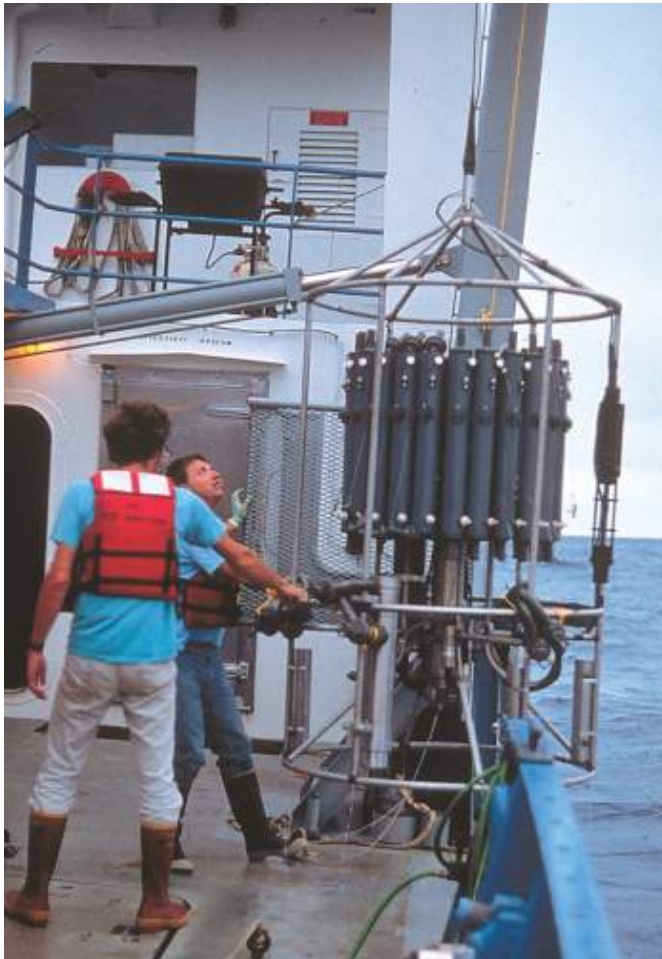
SeaTech transmissometer 25 cm path length
