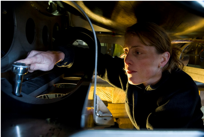
Installing electronics pressure housing racks
