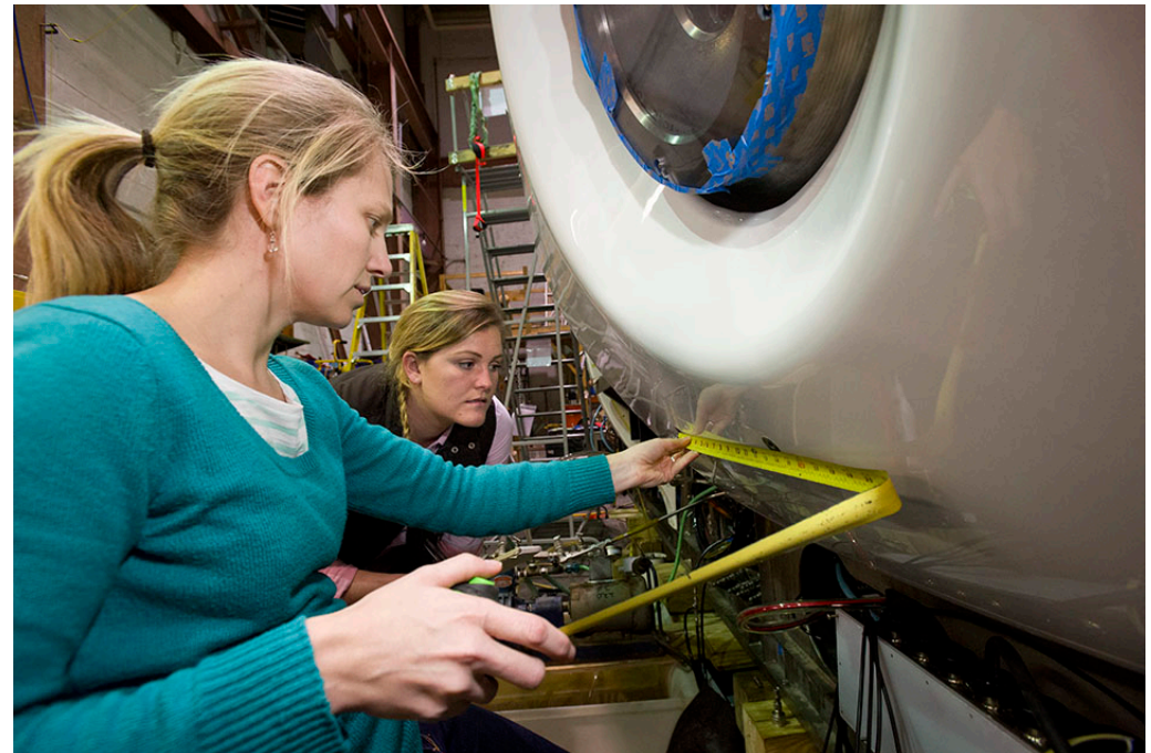
Measuring hole spacing for inserts (used for attaching lower skins) installed in the lower forebody foam block
