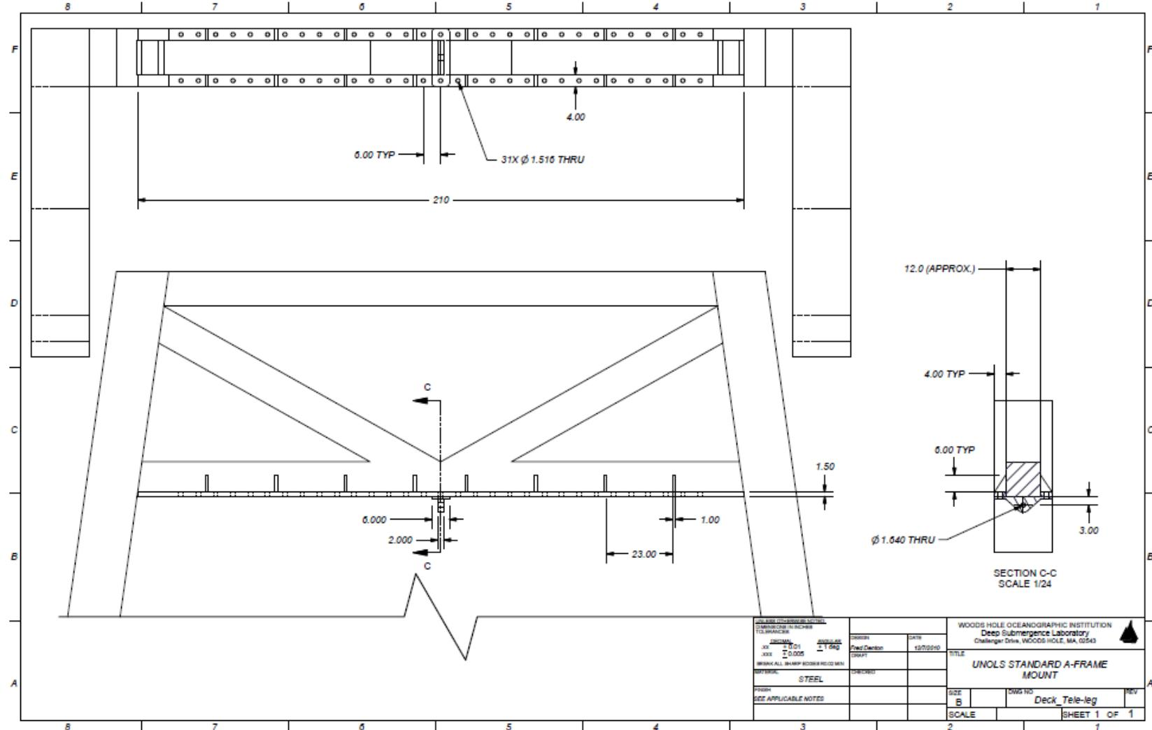
The standard bolting pattern shall be 6.00 inches between bolt hole centers athwartship and 16.00 inches between bolt hole centers fore and aft
