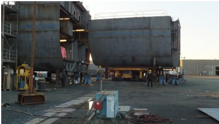
Lining Up Mod 3 with Mod 4
