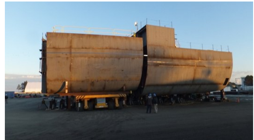
AGOR 28 Mod 3 & 4 ready for joining
