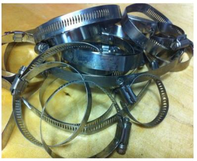
A hose clamp or hose clip is a device used to attach and seal a hose onto a fitting such as a barb or nib.
