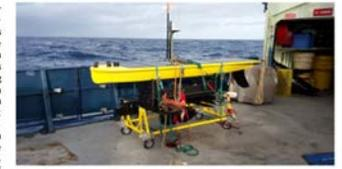
Fig. 1. LRI Wave Glider SV) configured as a communications relay. The hull on the “sub” houses a WHOI Micro Modem. One of the payload modules in the “float” contains a WHOI-designed Iridium modem/GPS receiver module that relays messages to and from the Micro Modem over Iridium as Short Burst Data (SDB). The relay functionality is decoupled from normal operation of the vehicle except for drawing power.
