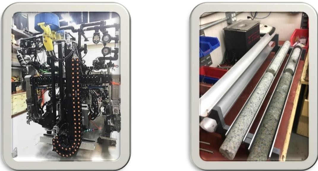
Figure 1: (Left) The multi-core drill system mounted to the front of ROPOS (minus the foam pack), and (Right) the selection of cores drilled in the test tank November 3-5, 2020 .
