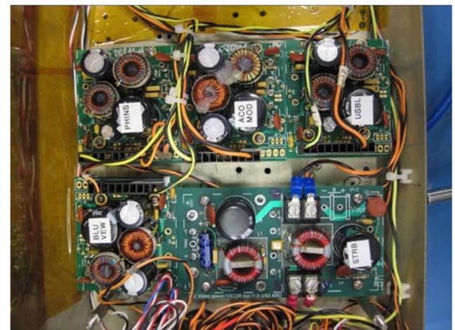
Existing DC/DC converters inside the main housing
