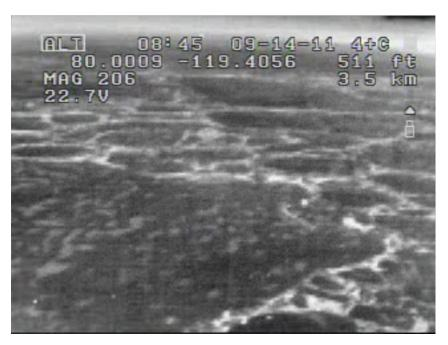
RAVEN UAS imagery used to find open water for launch and recovery of Canadian ISE AUV w multibeam
