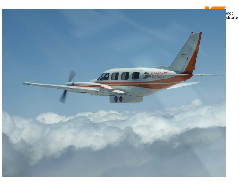
UTSI Flight Research Piper Navajo with NASA Marshal Airborne Polarimetric Imaging Radiometer (MAPIR) Under Fuselage Nacelle
