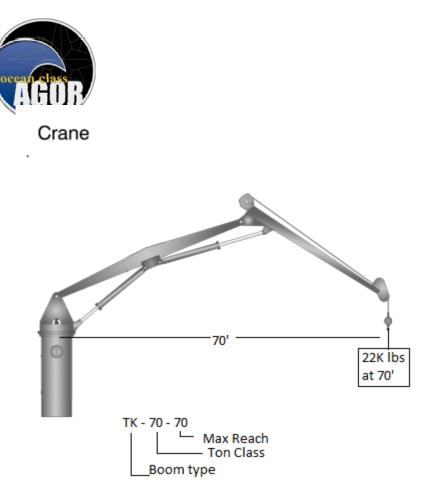
**K Series** - Knuckle boom cranes use hinged box section booms, optionally equipped with telescopic jib extensions. These models use one, two, or three main lift cylinders, and jib cylinders can be stowed horizontally to save space.
