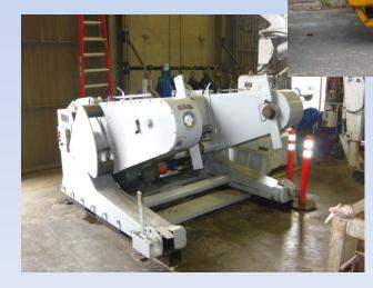
Note: all of this equipment is 1960's vintage: no capability for precise level winding or tensioning.
