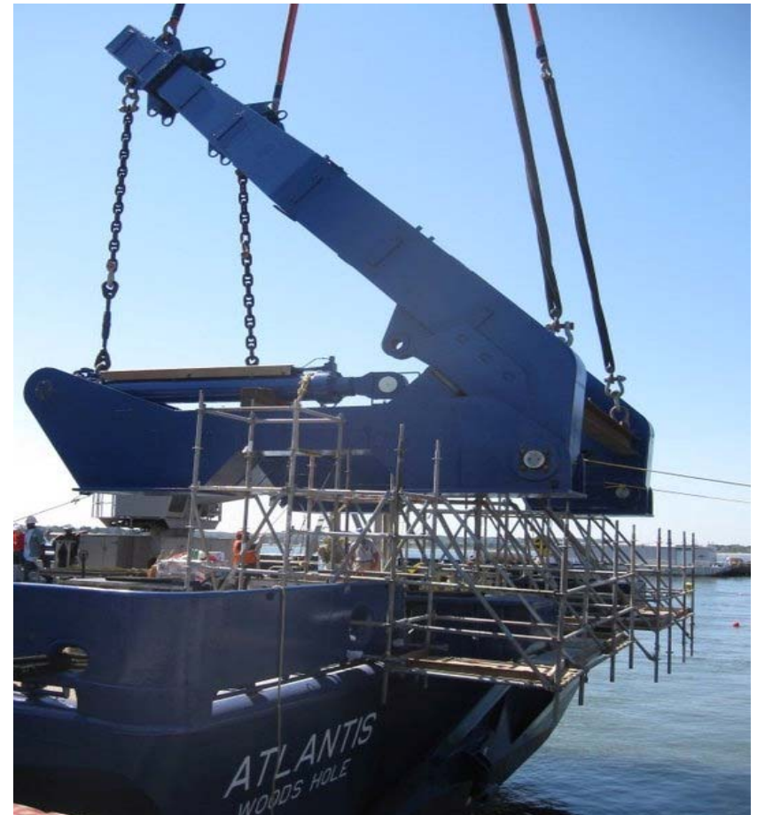
Installing the A-frame March 2011
