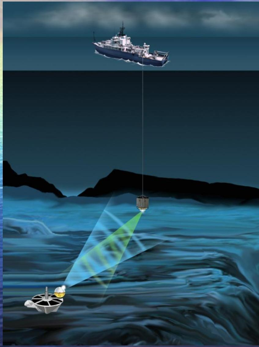
Wireless (optical) data transfer from seafloor instrument to surface vessel
