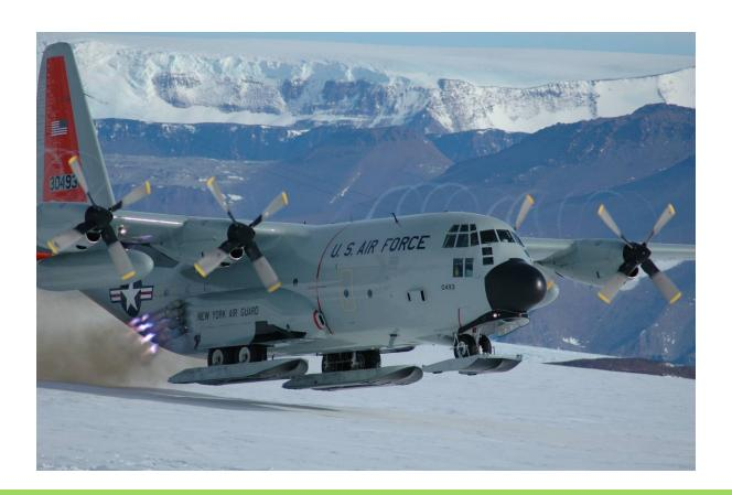
JATO assist for take off requires an estimated \$7M budget item each year; 8 bladed props and electronic propeller controls should eliminate the JATO requirement
